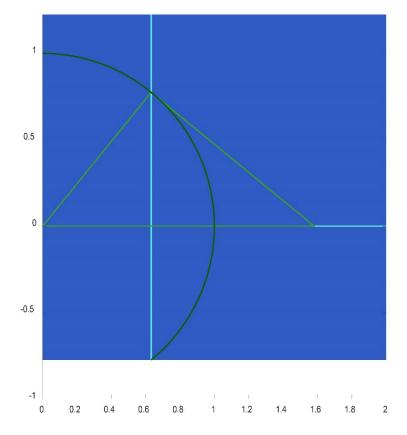
The angle at the top of the triangle is straight, as one side is a ray from the origin and the other is tangent to the unit circle which has its centre at the origin. This implies that the distance from the origin to the vertical muntin of the window is the reciprocal of the base of the triangle.
